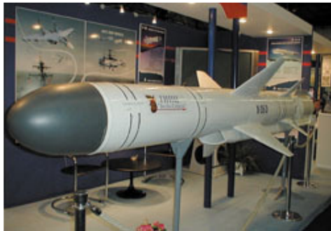
The Russian Kh-35 Uran (NATO: SS-N-25 Switchblade) is a medium-range anti-ship missile that entered service in the early 1990s and that closely resembles the US Harpoon (so much so that it was dubbed "Harpoonski" in Western circles). Like the Harpoon, it is deployable on a wide variety of platforms, with ship- and air-launched and coastal-defence versions available. Photo by Michael Puttré
