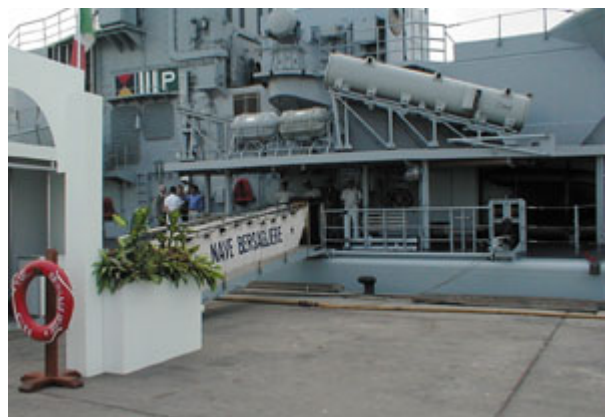
The Artigliere-class frigate Bersagliere of the Italian Navy during a port call to Abu Dhabi in March 2001. The ship, classified by the Italians as a fleet patrol ship, carries eight Otomat Teseo Mk 2 anti-ship missiles in four twin launchers. A twin launcher is visible above and to the right of the gangway. Photo by Michael Puttré
