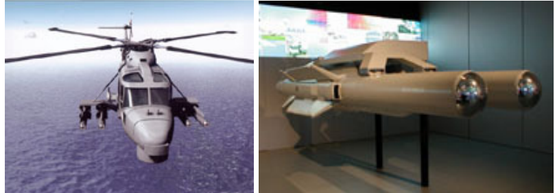
The MBDA Polyphem missile is a multi-purpose weapon with a camera in the nose that sends real time video to the operator and command guided by means of a fiber-optic line, making it impervious to jamming. It is designed for ground and naval combat at a range of between 30 and 60 km. The image at left shows a Lynx helicopter with four Polyphem missiles on individual launch rails; the photo on the right is a mock-up of a twin-rail configuration. MBDA image, photo by Michael Puttré
