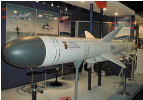
The Russian Kh-35 Uran (NATO: SS-N-25 Switchblade) is a medium-range anti-ship missile that entered service in the early 1990s and that closely resembles the US Harpoon (so much so that it was dubbed "Harpoonski" in Western circles). Like the Harpoon, it is deployable on a wide variety of platforms, with ship- and air-launched and coastal-defence versions available. Photo by Michael Putré
