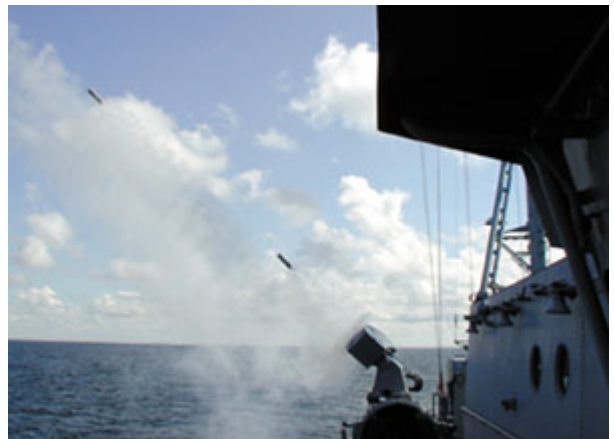
The Multi-Ammunition Softkill System (MASS) decoy launcher throws a pattern of dual-mode chaff and flare rounds from a German K-130 corvette. It can accommodate up to 32 rounds of varying types. The system deploys a tight decoy pattern close to the ship and is intended to counter supersonic and late-locking anti-ship missiles. Buck NT photo
