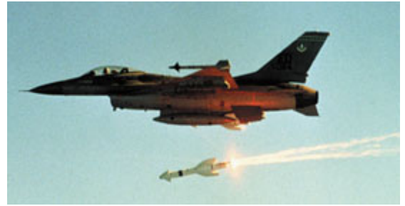
A US Air Force F-16 fires a Penguin 3 anti-ship missile. The first practical Western anti-ship missile, the Norwegian Penguin family is widely used and carried by a variety of fixed-wing aircraft, helicopters, and ships. In US service, the missile is designated AGM-119. US Air Force photo
