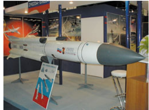
The Russian X-31 (NATO: AS-17 Krypton) air-launched anti-ship missile is derived from the Kh-31P anti-radiation missile. It has a booster-rocket motor and four solid-fuel ramjets attached around a cylindrical body, giving the missile excellent speed - exceeding Mach 3.6 - and a maximum range 110 km. Photo by Michael Puttré
