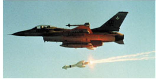
A US Air Force F-16 fires a Penguin 3 anti-ship missile. The first practical Western anti-ship missile, the Norwegian Penguin family is widely used and carried by a variety of fixed-wing aircraft, helicopters, and ships. In US service, the missile is designated AGM-119. US Air Force photo
