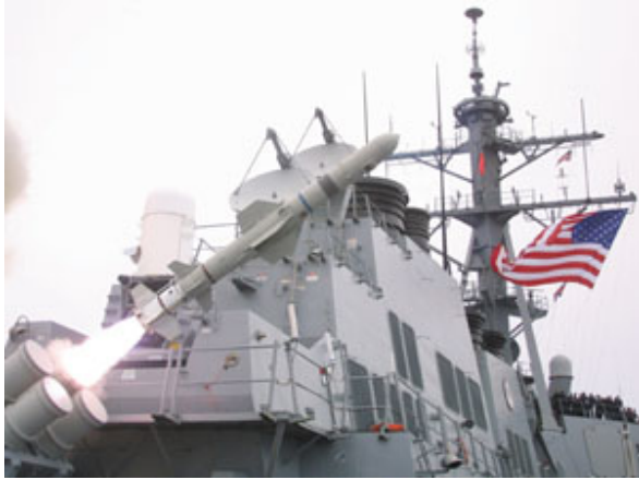
The first Boeing Harpoon Block II missile is fired from the USS Decatur , on June 7, 2001. Designed for littoral operations, the Block II missiles incorporate GPS guidance Harpoon Block II incorporates the inertial measuring unit from the Boeing Joint Direct Attack Munition (JDAM) program, and the mission computer and GPS receiver/antenna from the Boeing Standoff Land Attack Missile- Expanded Response (SLAM-ER), enabling it to execute both anti-ship missions and coastal-target suppression. Boeing photo
