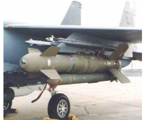
The AGM-130 stand-off weapon (shown here hung under an F-15E), was widely employed in the Kosovo air campaign. Its direct ancestor, the GBU-15 glide bomb, was used in small numbers in Desert Storm.
