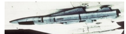
A definite heavy-hitter: a Kh-22 (AS-4) missile as carried under a Tu-22M bomber
