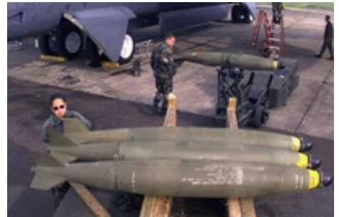
Mk-82 bombs being loaded on a B-52 prior to a strike mission
