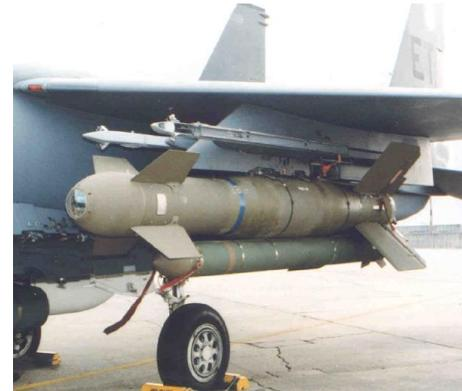
**The AGM-130 stand-off weapon (shown here hung under an F-15E), was widely employed in the Kosovo air campaign. Its direct ancestor, the GBU-15 glide bomb, was used in small numbers in Desert Storm.**
