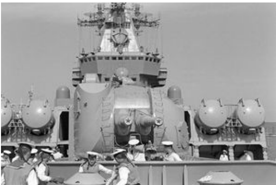
A view from the bow. The AK-130 gun mount and the foremost SS-N-12 launcher pairs are clearly visible. Notice also the fire-control director on top of the bridge
