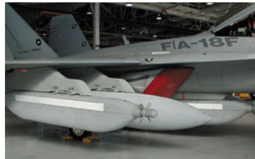
Boeing and its partner Northrop Grumman have funded development of the EA-18 airborne electronic attack concept aircraft, which they hope will be selected as a follow on to the EA-6B Prowler. The test configuration consists of a used F/A-18F Super Hornet leased from the Navy that carried three ALQ-99 physical mockups, including one low band pod mockup under the fuselage. Wingtip ALQ-218 receiver pods are still undergoing wind tunnel testing. To support the effort, Boeing had developed an advanced EA-18 cockpit simulator to demonstrate interface and workload for the two-place crew. Photo by Michael Puttré
