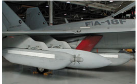
Boeing and its partner Northrop Grumman have funded development of the EA-18 airborne electronic attack concept aircraft, which they hope will be selected as a follow on to the EA-6B Prowler. The test configuration consists of a used F/A-18F Super Hornet leased from the Navy that carried three ALQ-99 physical mockups, including one low band pod mockup under the fuselage. Wingtip ALQ-218 receiver pods are still undergoing wind tunnel testing. To support the effort, Boeing had developed an advanced EA-18 cockpit simulator to demonstrate interface and workload for the two-place crew. Photo by Michael Puttré
