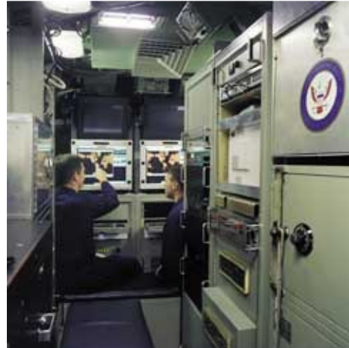
The Lockheed Martin ASTECS (Advanced Submarine Tactical ESM Combat System) or AN/BLQ-10, for the Virginia-class integrates threat warning and intelligence gathering, as well as sufficiently good direction-finding for anti-ship and land-attack missile targeting. It may be backfitted to the Seawolf-class (to replace the AN/WLQ-4) and perhaps to some Los Angeles-class vessels. (US Navy photo)
