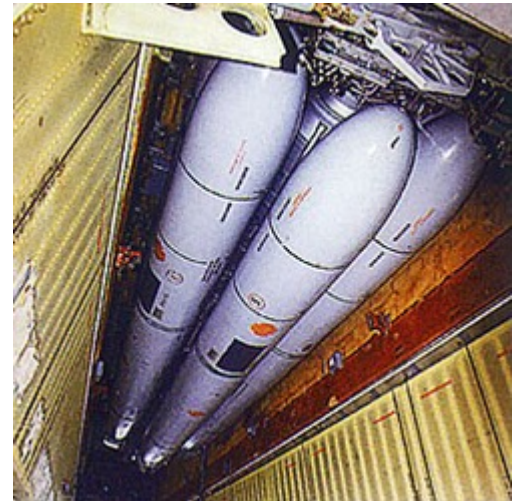
Kh-55 missiles in the internal rotary launcher
