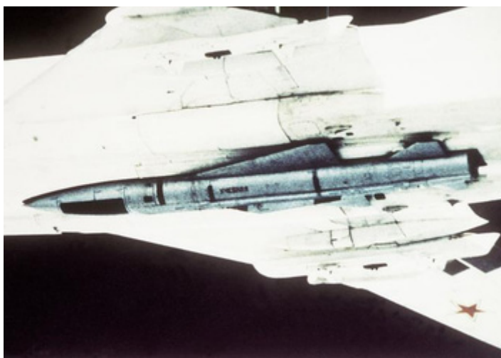
A Kh-22PSI is carried semi-recessed on the fuselage of a Tu-22M2
