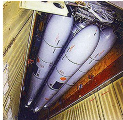
**Kh-55 missiles in the internal rotary launcher**
