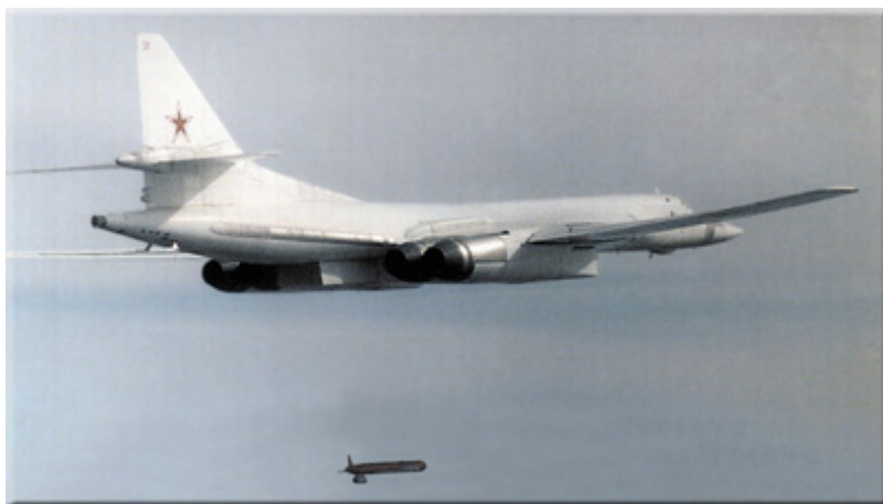
A Tu-160 releases a Kh-55 cruise missile during trials
