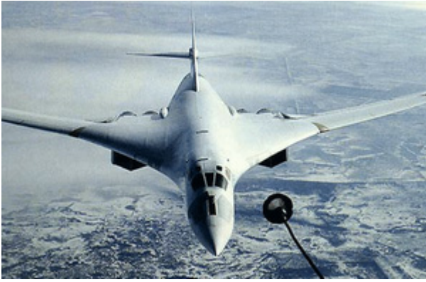
A Tu-160 approaches the drogue of an Il-78 for a mid-air refuelling sequence
