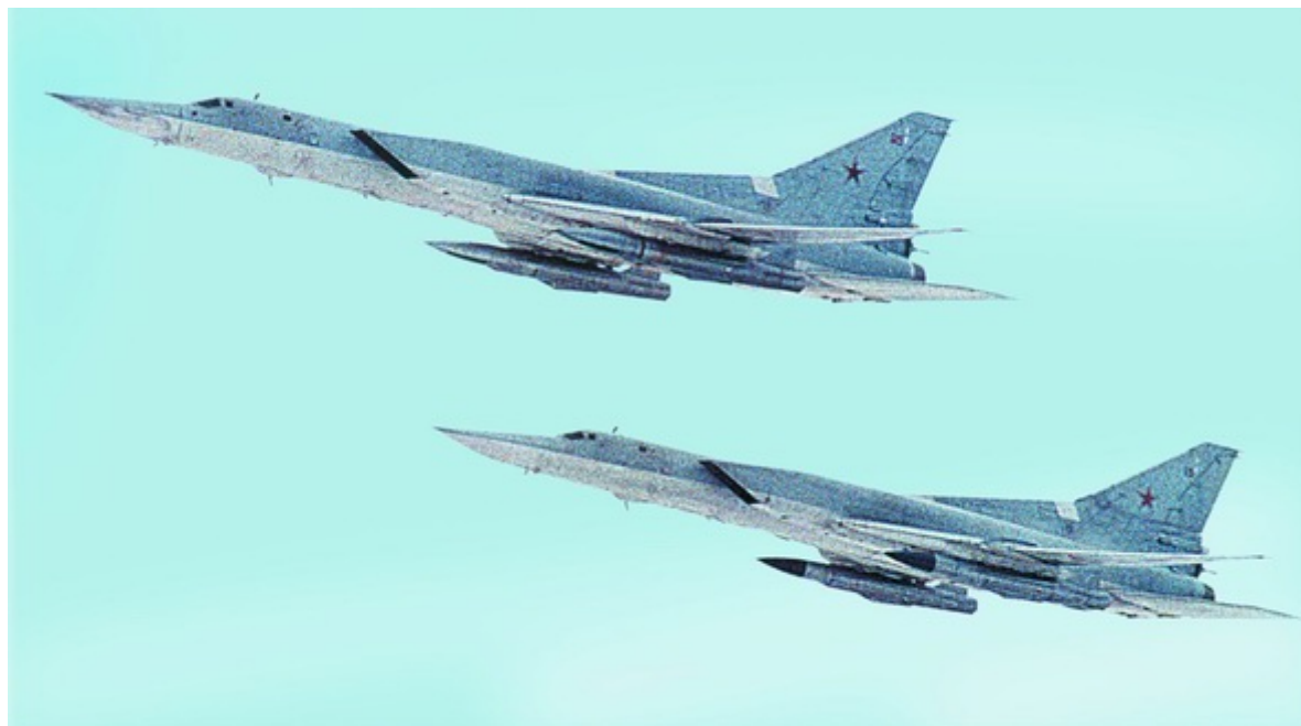
A pair of Tu-22M3s demonstrate a typical operational medium/long-range load of two Kh-22s each. Notice the different radomes on the missiles: The upper pair is probably an inertial land-attack version (the very slim downwards-facing opening is the window for the altimeter radar). The lower pair is the anti-ship version.
