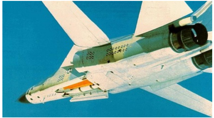
The FB-111 could carry six SRAMs or thermonuclear bombs; four under the wings and, as this test flight demonstrates, another two in the fuselage weapons bay
