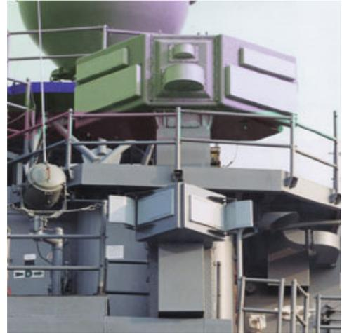
**The AN/SLQ-32(V)5 installation on US Oliver Hazard Perry-class frigates consists of the SLQ-32(V)2 passive ESM array (above) and the Sidekick active jammer (below). The Sidekick was developed in a crash six-month program after the USS *Stark* was hit by two Iraqi Exocet missiles in May 1987. The existing SLQ-32(V)3 system with an integral active jammer was too heavy for the class. Raytheon photo**
